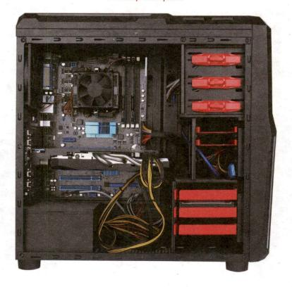
**Motherboard:** The motherboard is the main board that is screwed into the computer case directly. Its function is to connect all the components so that they may communicate and work together.
